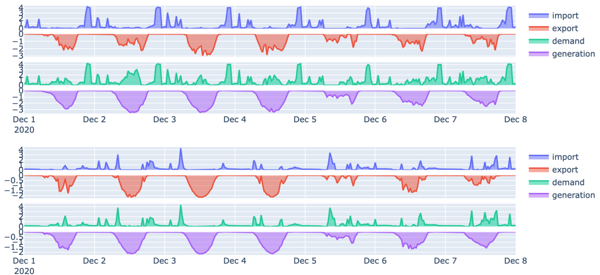
Figure 9. Examples of conversion of import/export to demand/generation for two different NMIs
