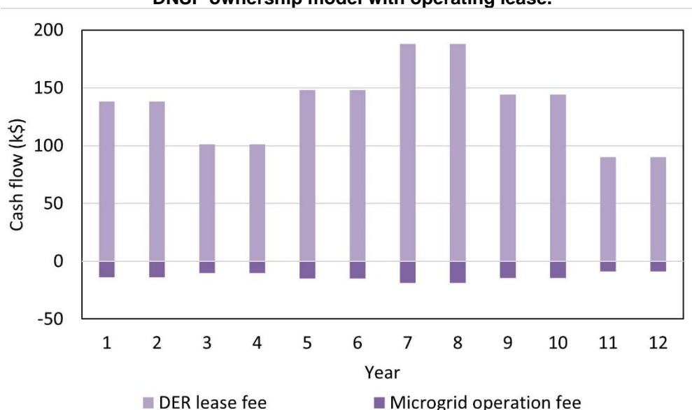
Figure 103. Zoom over the 12 years operation of the microgrid of the resulting cash flows, i.e., benefits (+) and costs (-), for the “DNSP” actor under a DNSP ownership model with operating lease, excluding the DER CAPEX and salvage value financial flows.
