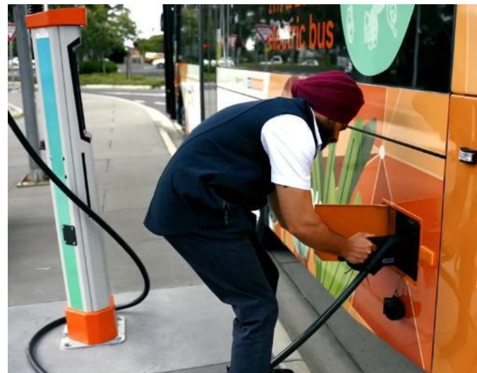
Plug-in charger at Monash University for top-up at layover – same charger as used at the depot
