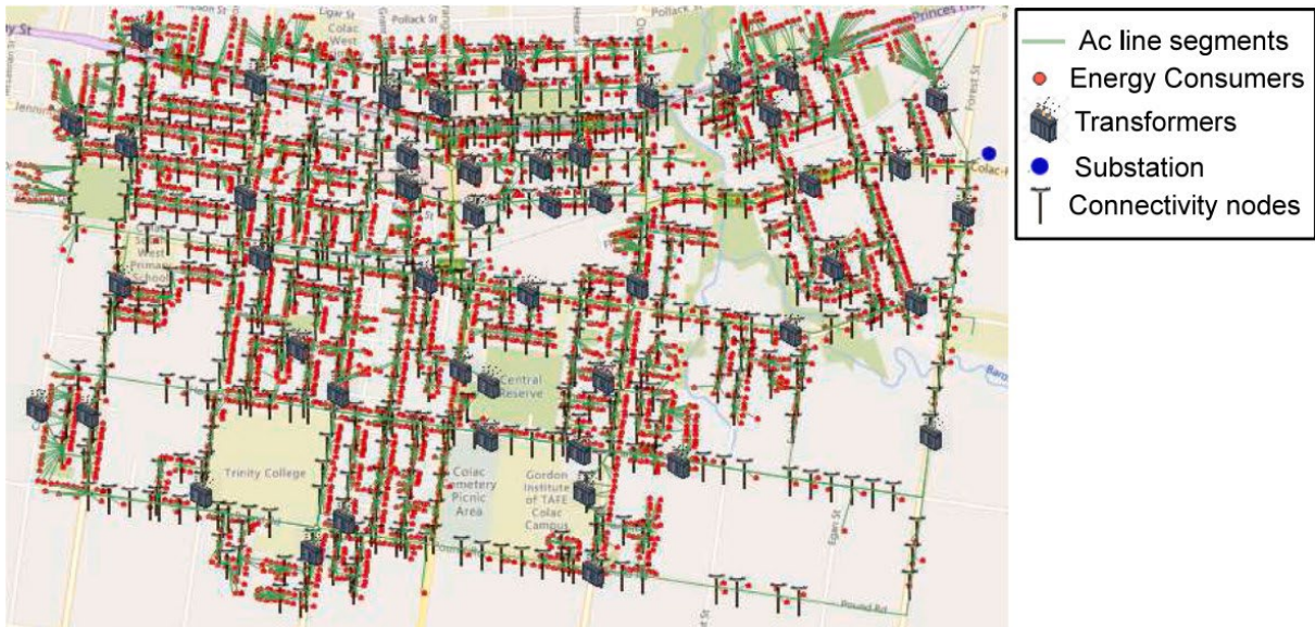
Figure 6: Illustration of a synthetic distribution network for Colac region in Australia [2].
